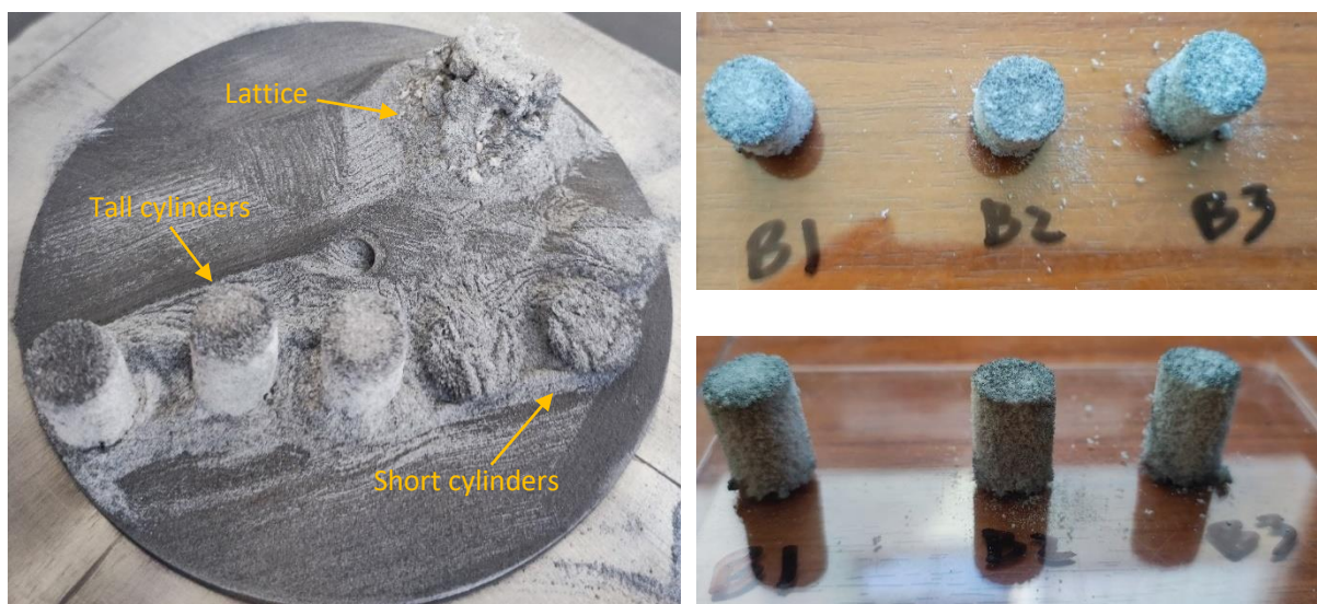
Figure 6.11: HA10G printed samples. Printing bed post the depowdering step (left), tall cylinder top (upper right) and side (lower right).
