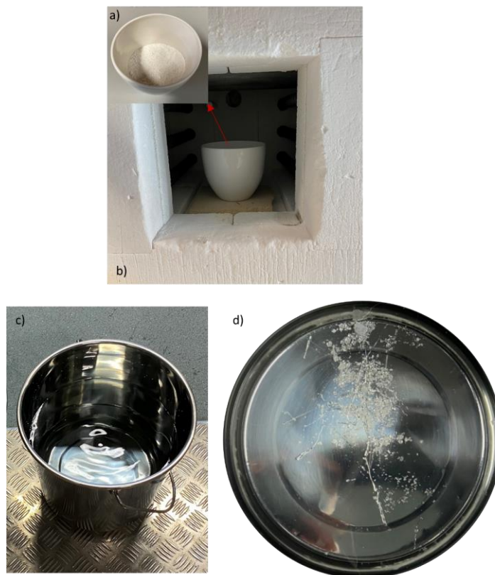
Figure 4.1: Overview of the glass making process. a) Powder reagents in porcelain crucible, b) Porcelain crucible placed within the furnace, c) Quenching tank filled with deionised water and d) Glass frit.
