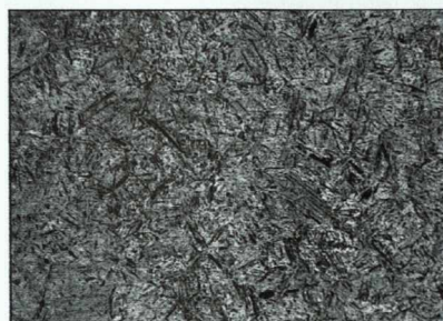
Position 2: T= 710°C No bulk ferrite present. Decarburised zone ferrite forms.
