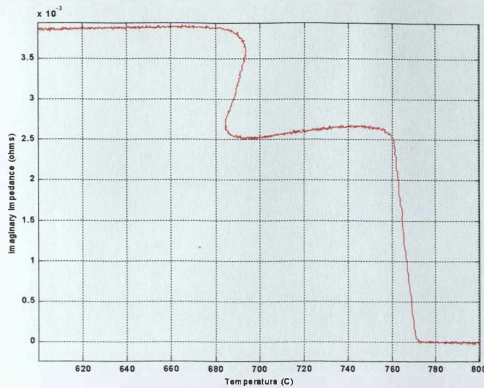
Figure 5.26: Impedance – temperature response for vacuum homogenised high carbon steel after one heating cycle at a frequency of 2Hz.
