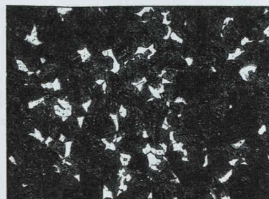
Position 4: T= 690°C 9 % bulk ferrite.
