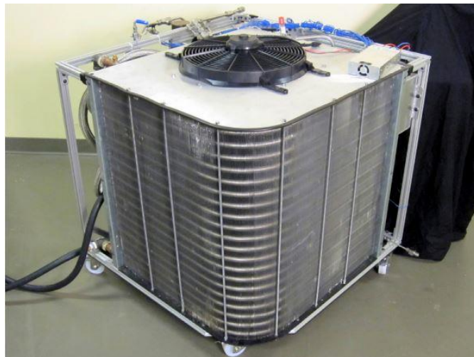
Figure 2-12 : Compact \text{NH}_3\text{-H}_2\text{O} VARS developed by Staedter and Garimella [46].
