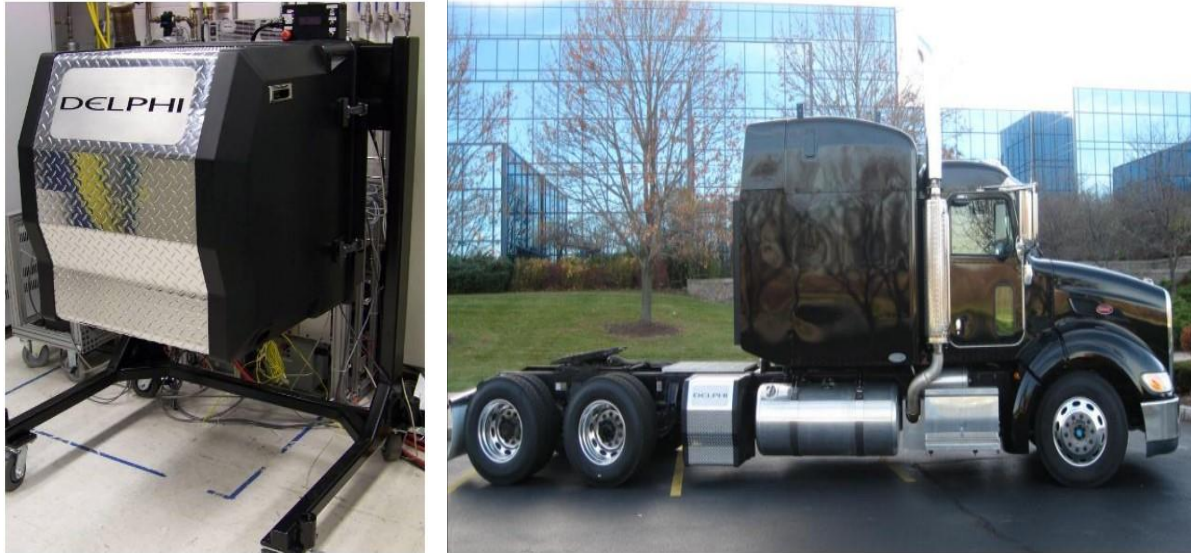
Figure 2-6 : 3.5 kW SOFC APU developed by Delphi automotive system [34].
