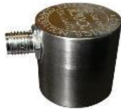
Figure 5-4: AE sensor R50 \alpha (MISTRAS, 2011b).
