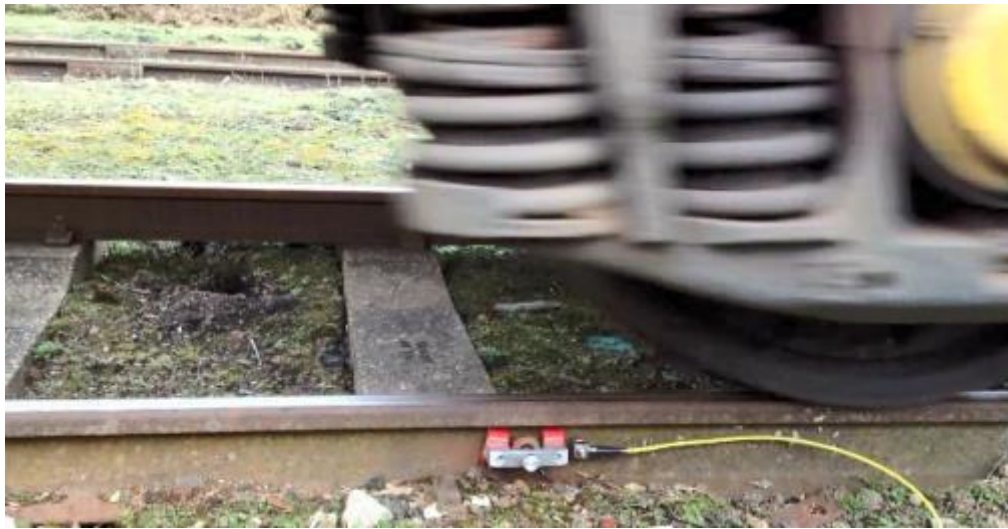
Figure 6-9: Wayside accelerometers and AE sensors.
