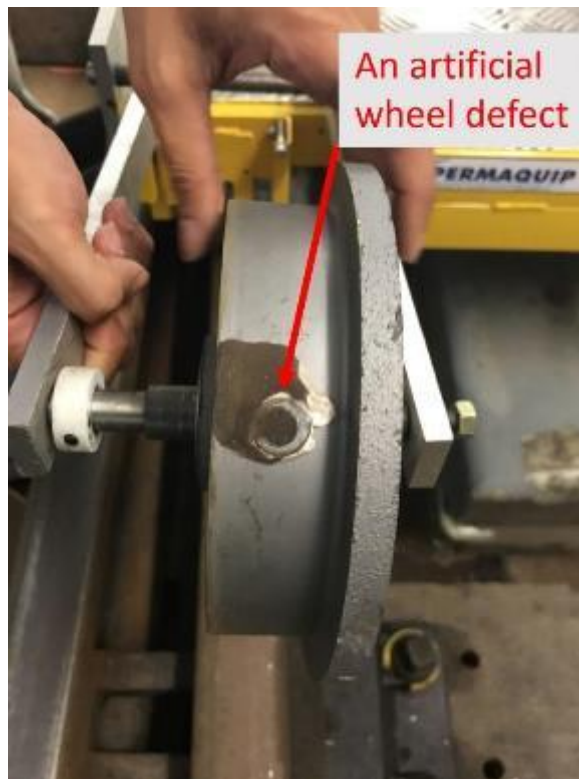
Figure 5-22: A faulty wheel used in the trolley.
