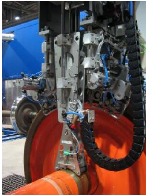
Figure 3-9: Probe system carriers for wheel and axle inspection by GE company (Kappes et al., 2007).
