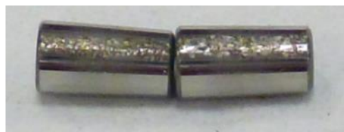
Figure 5-28: Rollers with artificial defects.
