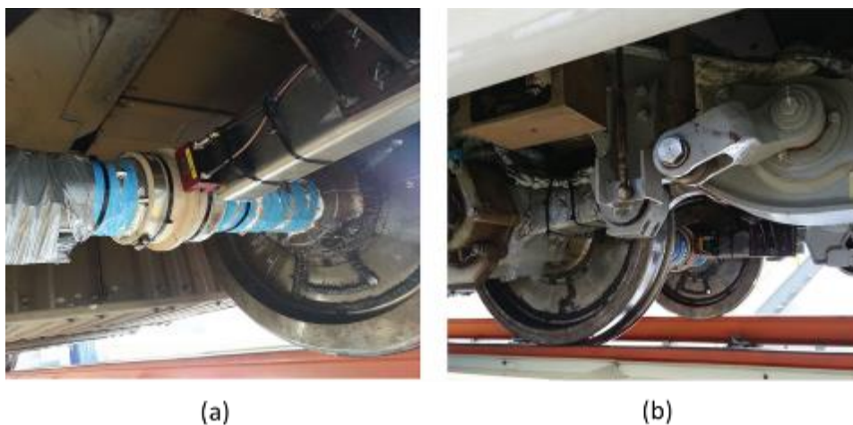
Figure 3-33: The wheels mounted under high-speed train model CRH6 in China (a) antenna unit (b) instrumented wheelset (Jin, 2020).
