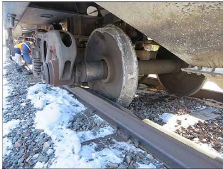
Figure 1-4: The manufacturing defects of the wheel cause the derailment in Canada (Transportation Safety Board of Canada, 2015).
