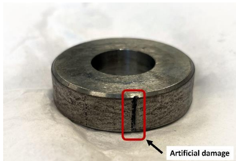
Figure 5-30: A damaged EN24T sample.
