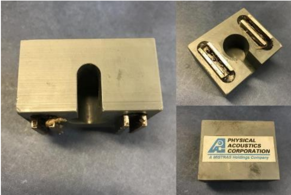
Figure 5-24: A magnetic adapter for the placement of AE sensor on the wayside measurement.
