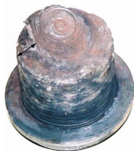
Figure 2-14: The missing piece of the axle due to the deformation along the circumference
