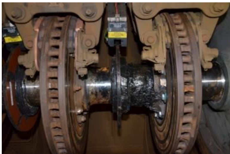
Figure 3-32: Specially designed auxiliary brackets for wireless signal transfer system (J. Wang et al., 2021).
