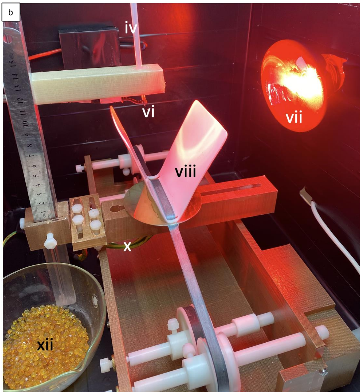
Figure 3.2.5 (a) Schematic illustration and (b) photograph of the custom-designed spooling set-up for continuous producing aligned nano-fibres using a Vee-shield collector: (i) solution dispensing unit; (ii) syringe; (iii) electro-spinning chamber; (iv) PTFE tube; (v) positive terminal; (vii) IR lamp; (viii) Vee-shield collector; (ix) high-voltage power supply; (x) ground wire; (xi) winding motor; (xii) silica gel; and (xiii) tape winding rig.
