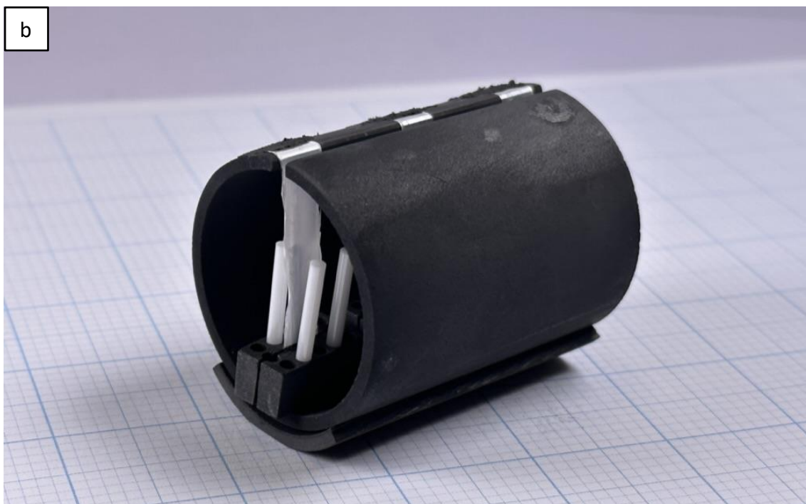
Figure 3.3.4 Photograph of (a) weight rods made of zirconia, tungsten carbide and alumina and (b) the assembly of nano-fibre loaded on the graphite fixture with four alumina weights.
