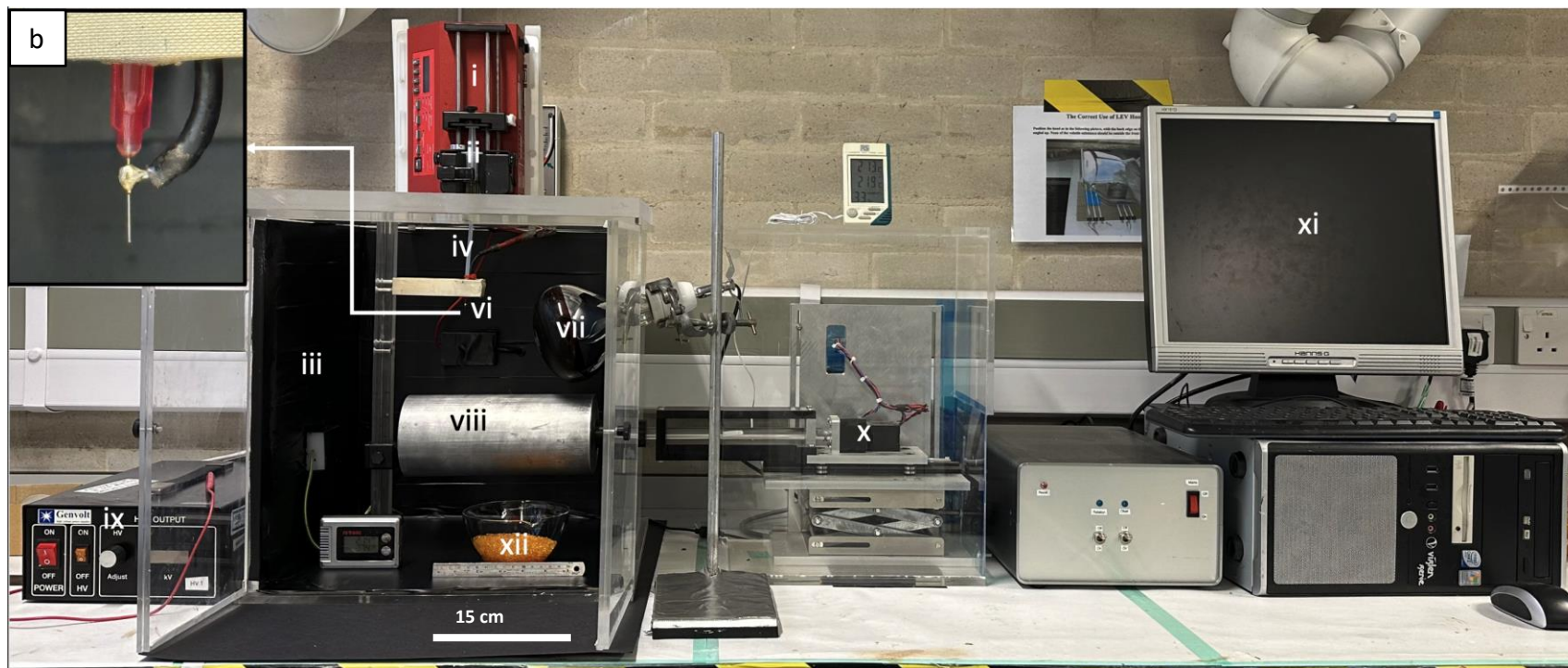
Figure 3.2.3 (a) Schematic illustration and (b) photograph of the rotating mandrel set-up for producing randomly oriented PAN nano-fibres: (i) solution dispensing unit; (ii) syringe; (iii) electro-spinning chamber; (iv) PTFE tube; (v) positive terminal; (vi) needle; (vii) IR lamp; (viii) rotating mandrel; (ix) high-voltage power supply; (x) electric motor; (xi) computer; and (xii) silica gel. The insert in Figure 3.2.3 (a) shows a transparent view of the ground connection between the wire (green) and the inner surface of the mandrel. The insert in Figure 3.2.3 (b) shows a magnified view of the connection between the needle and the positive terminal of the power supply.
