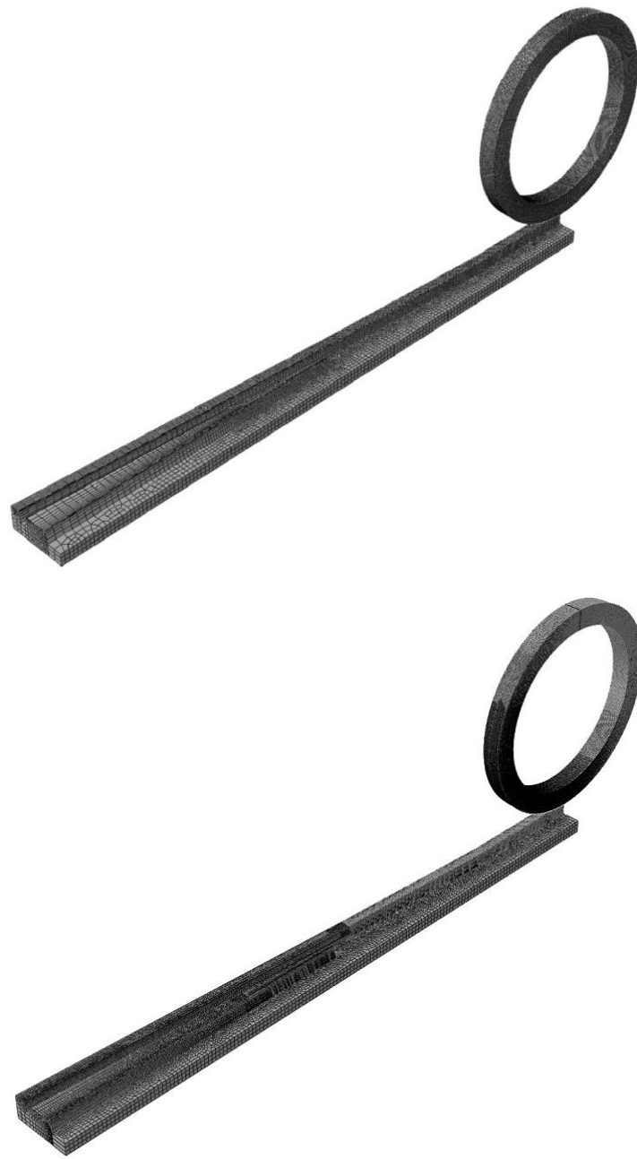
Figure 4.3 8 mm (upper) and 2 mm (lower) mesh models.
