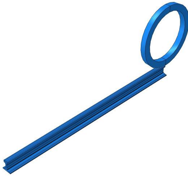
Figure 5.29 Model of wheel-rail dynamic interaction.
