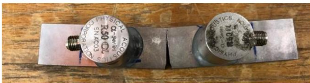
Figure 5.28 The R260 specimen after failure from the three-point bending fatigue test mounted with two AE probes [170].
