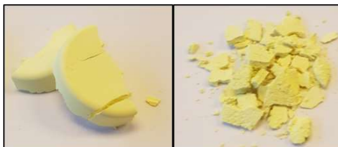
Figure S15. Fracture of CAN-Y Ar -T 8
