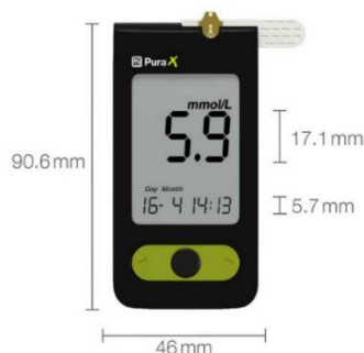
Figure 1.5. A portable mylife Pura X blood glucose meter [31].
