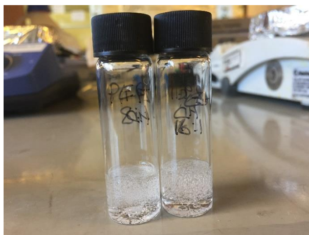
Figure 3.2. 2 mL gels of 15% PEGMEA-480:PEGDA-10,000 at a ratio of 8:1 (left) and 16:1 (right).
