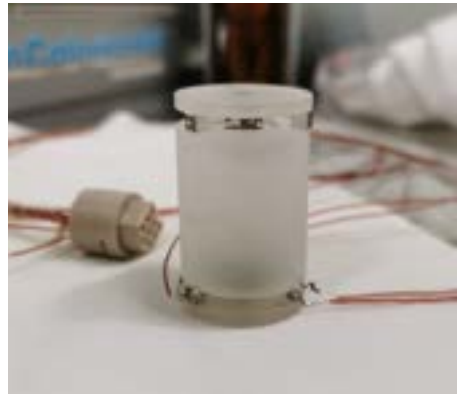
Figure 29: Fully assembled 2.6\mu\text{m} , ULE-FS tunable cavity.
