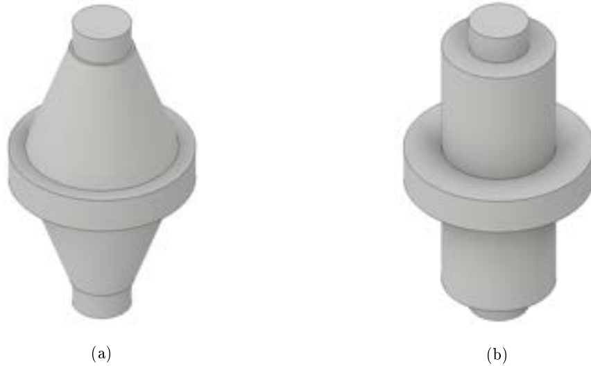
Figure 45: The CAD designs for both types of vertical cavities initially tested, with (a) double cone shape and (b) cylinder shape.
