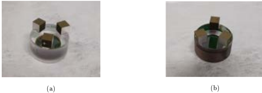
Figure 25: Both FS mirror's for the 2.6\mu\text{m} cavity with three piezo-chips evenly attached to the back of the mirrors, with (a) being plane-planar and (b) plane-concave with a radius of curvature of 500mm.
