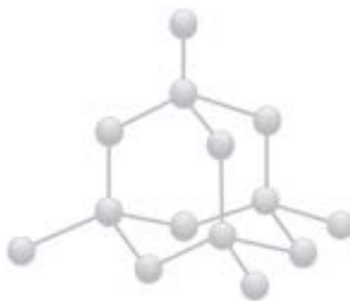
Figure 71: Diamond's tetrahedral structure, formed with carbon-carbon covalent bonds.
