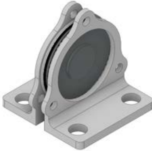
Figure 95: Initial CAD design for the support structure for diamond-diamond cavity, where the cavity is dark grey, the viton o-rings are black and the aluminium support structure is light grey.
