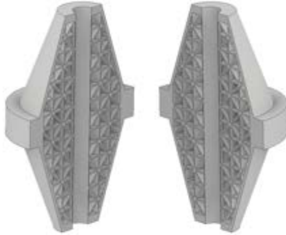
Figure 63: Final CAD design for the lattice spacer, in two halves to display the internal lattice.
