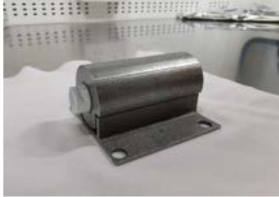
Figure 41: Image of the fully constructed hemispherical invar cavity, ready for testing.
