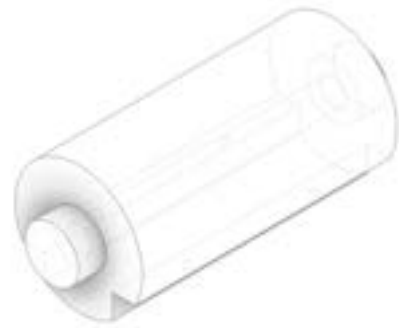
(b) A cylinder design with two square cut-outs, to create a "mushroom" shape.
