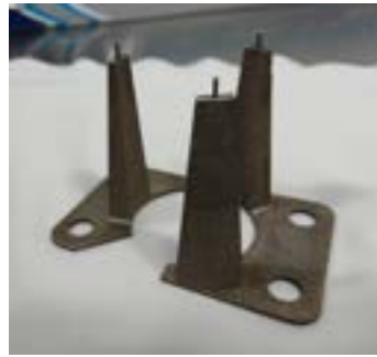
Figure 65: Final printed lattice support structure using SLM as discussed in Chapter 5.2.
