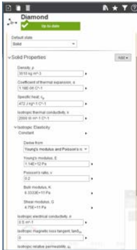
Figure 102: Values for the properties of diamond from the stock materials library in ANSYS.
