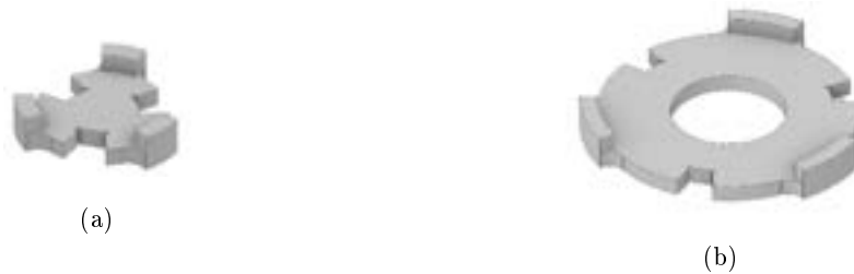
Figure 97: CAD designs for 3D printed parts to align the piezo's for the 2.6\mu\text{m} cavity, (a) for the FS mirrors and (b) for the ULE rings.
