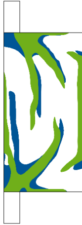
Figure 6.11 Comparison of the optimized flow channel designs for sieve reactors, green colour, and cylindrical reactors, blue colour, for fixed values of seeding parameters, level 1.
