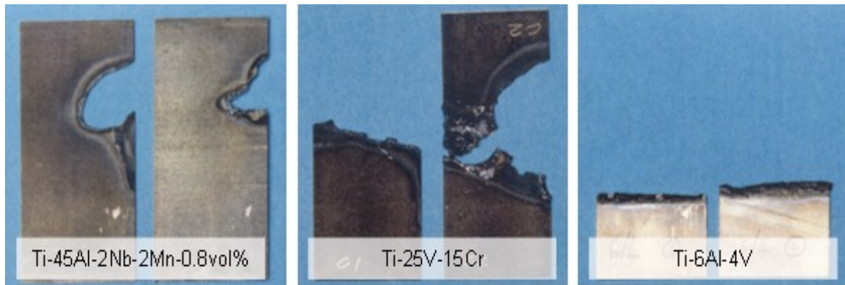
Figure 1.3: Comparison of burn resistance between different titanium alloys using 1x25x50mm coupons at 300°C, 695kPag air pressure and 150m/s air velocity [4]
