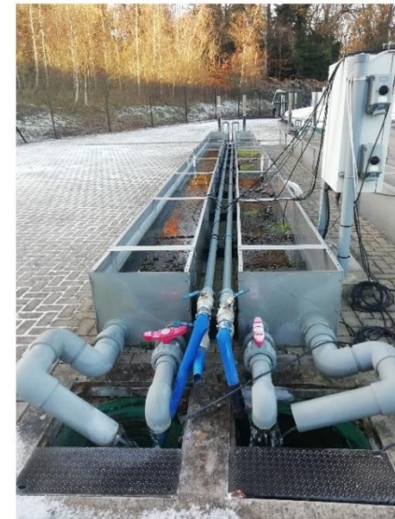
Fig. 2.9. Environmental Change Outdoor Laboratory (EcoLaboratory) at University of Birmingham. The EcoLaboratory is equipped with a range of semi-recirculating flumes (top). This study used 16 stainless-steel flumes (top right), which are groundwater-fed by a system of taps (bottom middle). Discharge and water depth are controlled by an outlet system (bottom right) and the number of pumps connected (bottom left and middle).
