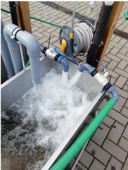
Fig. 2.9. Environmental Change Outdoor Laboratory (EcoLaboratory) at University of Birmingham. The EcoLaboratory is equipped with a range of semi-recirculating flumes (top). This study used 16 stainless-steel flumes (top right), which are groundwater-fed by a system of taps (bottom middle). Discharge and water depth are controlled by an outlet system (bottom right) and the number of pumps connected (bottom left and middle).
