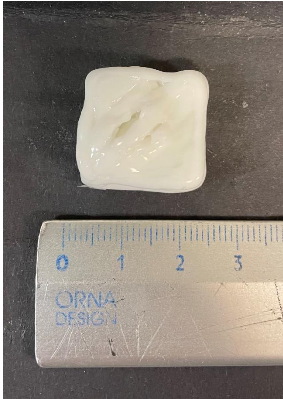
Figure 6.6 - A defective soy wax capsule manufactured using the freeze dropped method. Scale is in centimetres.
