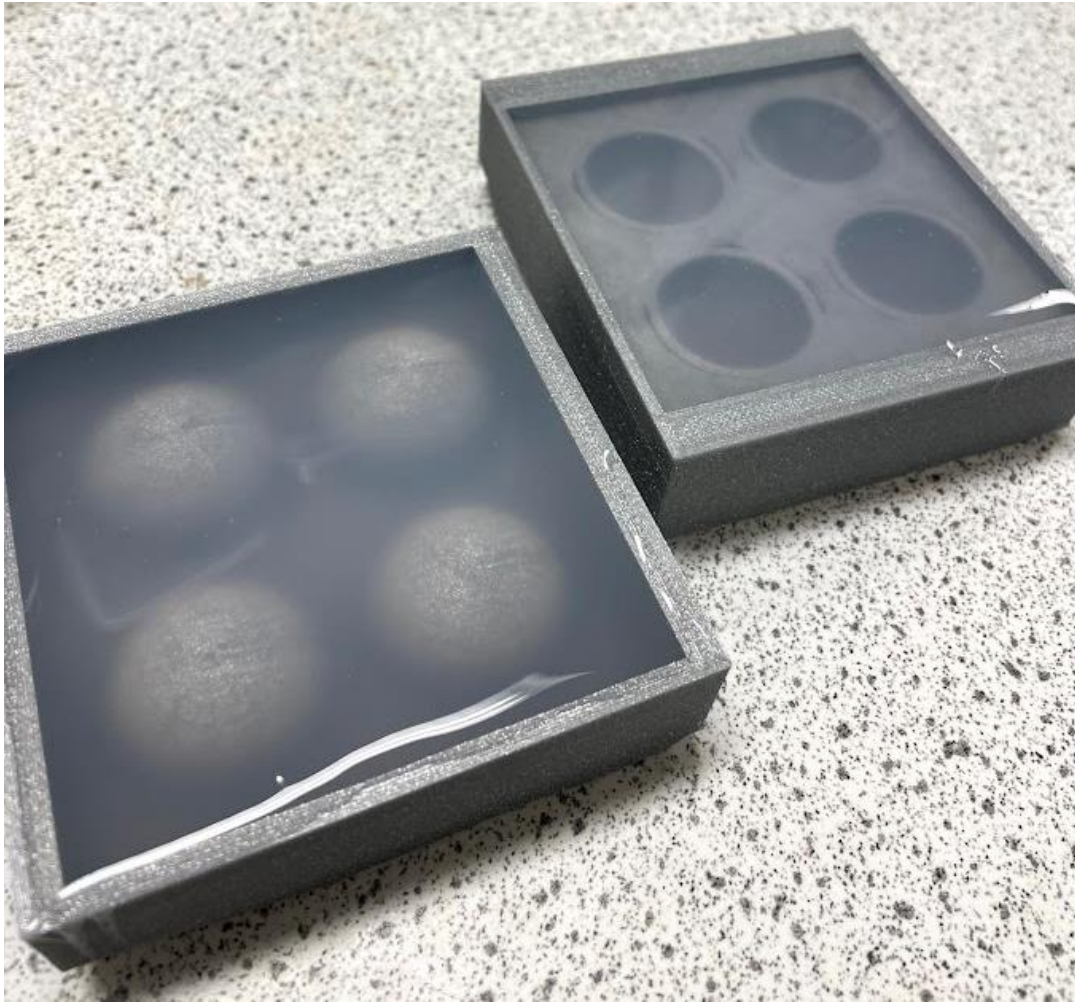
Figure 6.1 - Negative 3D printed moulds required for manufacturing capsules using the moulding method.
