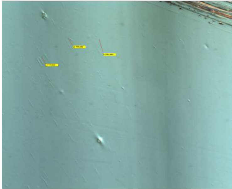
Figure 78: Optical Microscopy image of Scuffing defect taken with Zeiss light microscope. Length labels read 0.1 mm, 0.1 mm and 0.2 mm respectively left to right. Marker pen at top right is to help the surface focus.
