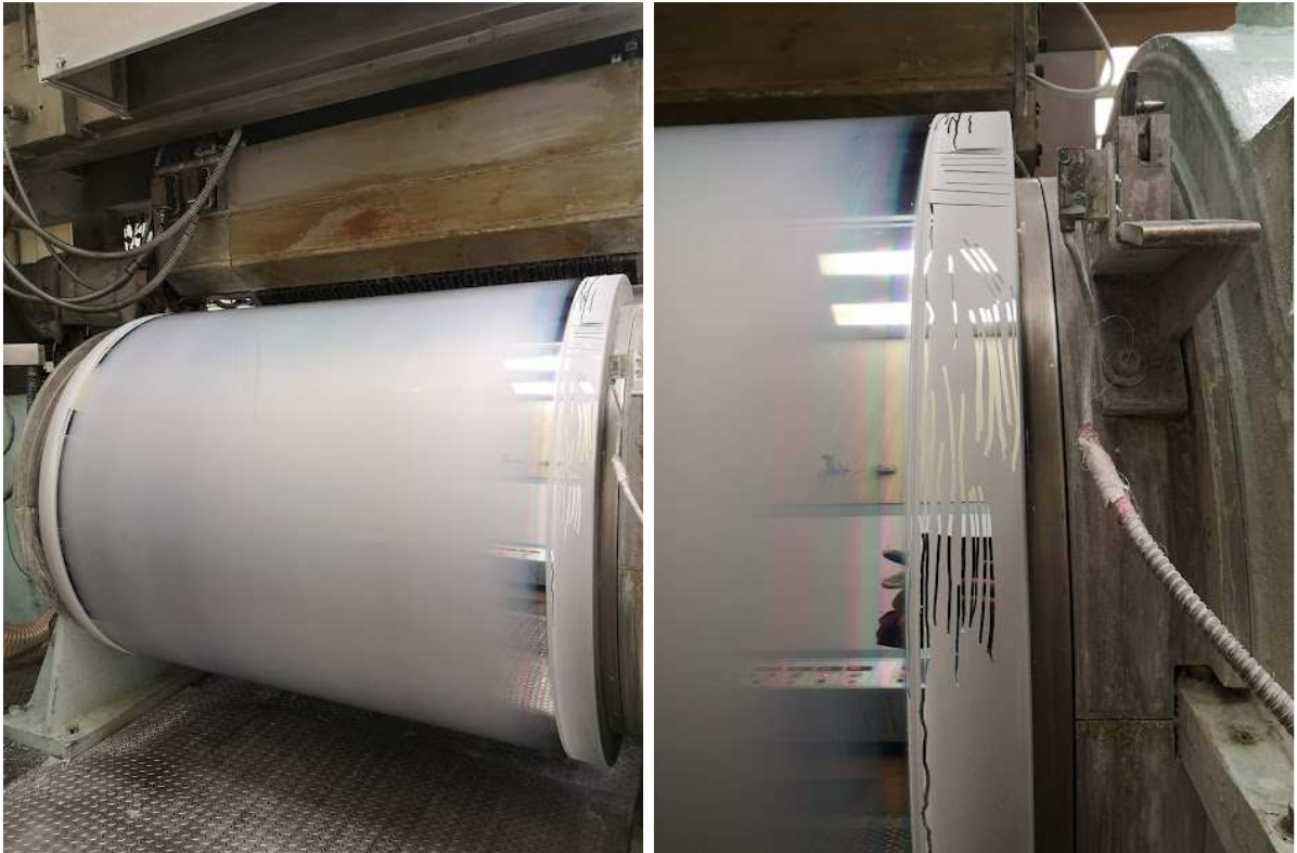
Figure 36: Photos of the casting drum from D52 production line with white powder build up at the edges and the centre portion obscured by condensation. Samples of powder have been removed leaving clean areas of the mirror-finish exposed.
