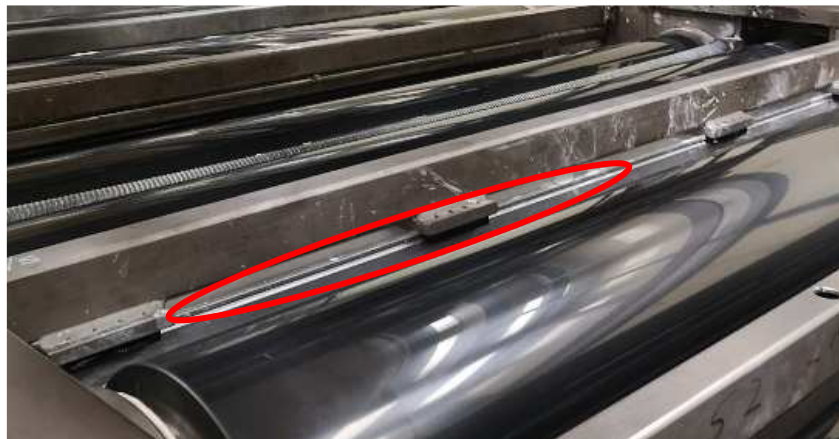
Figure 48: Photos of D52 forward draw. Area where FWD adjacent sample collected from metal work shown in red.
