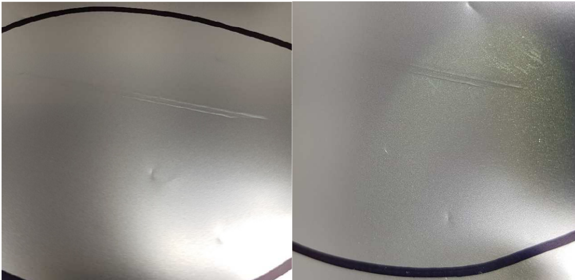
Figure 74: Replication scratches found on D52 film. Scratches appear identical in shape and form and were found at a specific separation distance.
