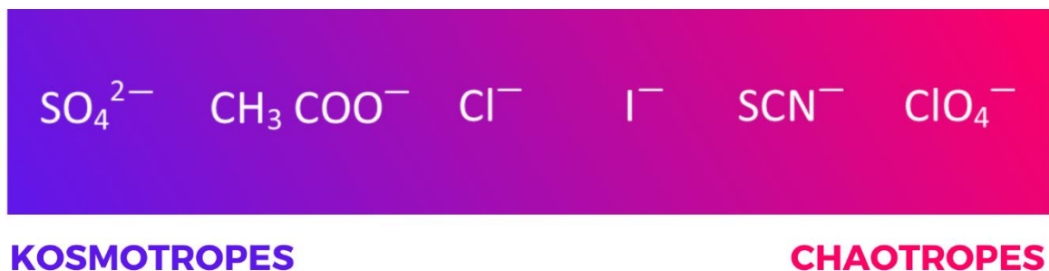
Figure 1.2 Hofmeister series for selected anions. Kosmotropic anions are situated to the left of the Hofmeister series, with chaotropic ions positioned on the right. \text{Cl}^- anions are known to be borderline kosmotropic.
