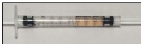
Figure 4.1 1 mL cropped syringe used a mold for 3D collagen gels.
