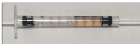
Figure 2.2 Cropped syringe used as mold for 500 \mu\text{L} collagen gels.
