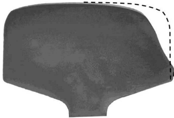
Figure 2.3 Example of tongue lipping on the contact surface of the rail head. The approximate original geometry is shown by the dashed line (Schilke, 2013).
