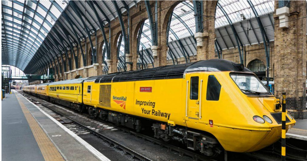
Figure 1.6 Image of the flagship new measurement train used by Network rail to monitor the structural health of the rail network (New Measurement Train (NMT) - Network Rail, 2022).
