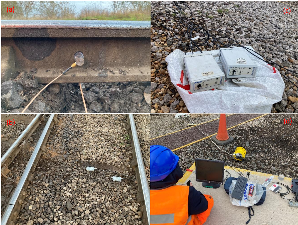
Figure 2.11 Images of the AE acquisition equipment used during field trails. (a) R50 \alpha AE sensors attached to rail web (b) pre-amplifier in rail bed (c) Amplifiers (d) Recording computer.
