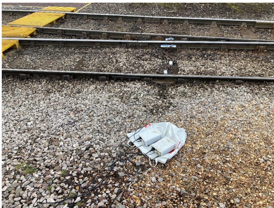
Figure 2.12 Image of the AE sensors, pre-amplifiers, and amplifiers in situ.
