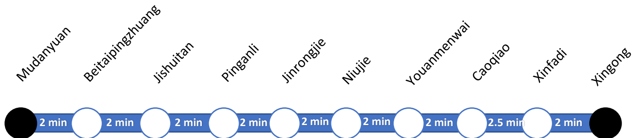
Figure 4-13 Planned running time between stations
