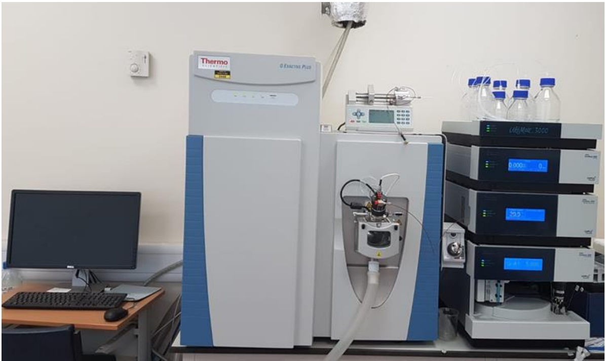
Figure 2-8 Thermo Q-Exactive Plus Orbitrap MS platform used for analysis of samples.
