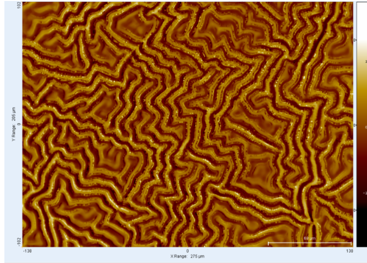
Figure 4.9: Interferometer image of the surface of planar PDMS coated with PVA in ambient.
