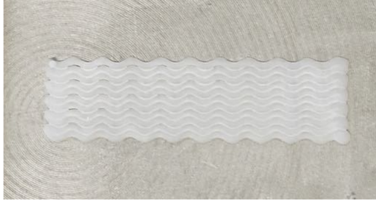
Figure 5.6: Example sample printed with a sine wave toolpath and 100% infill. Note the print defects present in some places between filament strands. Sample is 20 mm in length.
