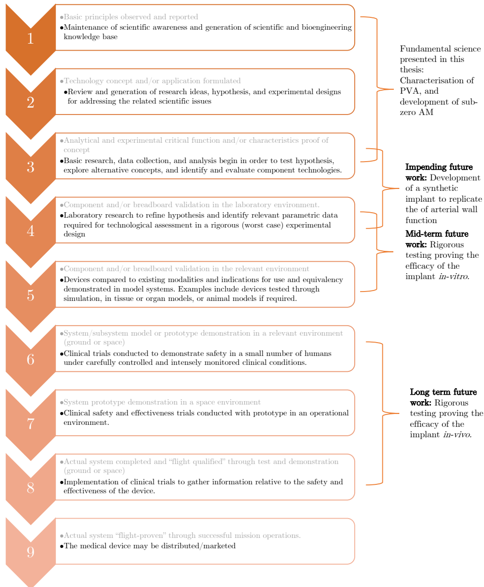
Figure 6.1: The original TRL system developed by NASA (grey), and the biomedical engineering equivalent (black). The example of an arterial wall replacement is shown on the right.
