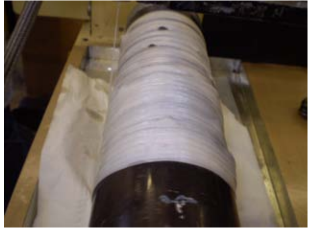
Figure 13 Photograph to show the as received waste slittings wound on to the mandrel.
