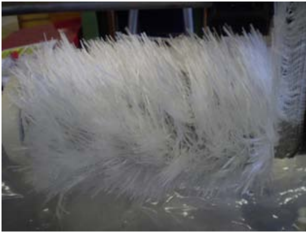
Figure 18 show the hedge hog appearance of the first layer of DLW has been wound.
