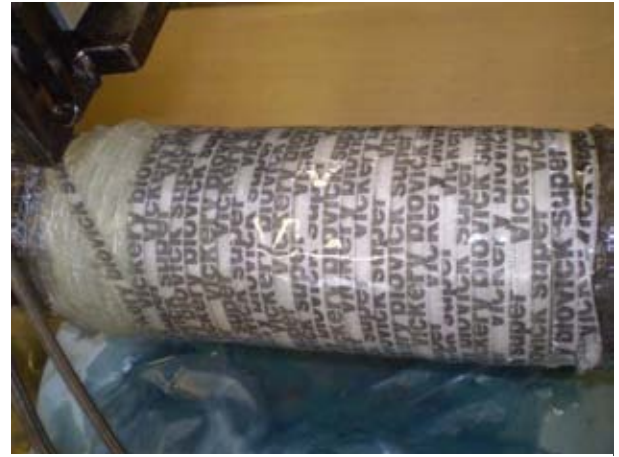
Figure 31 Photograph to show the outer layer of waste slittings as it was applied to two layers of the DLW.
