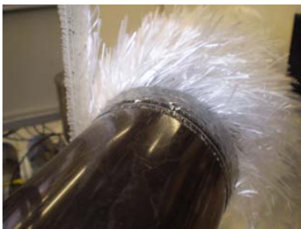
Figure 42 photograph showing the first layer of DLW being applied to the rotating mandrel. The loose ends are clearly visible.
