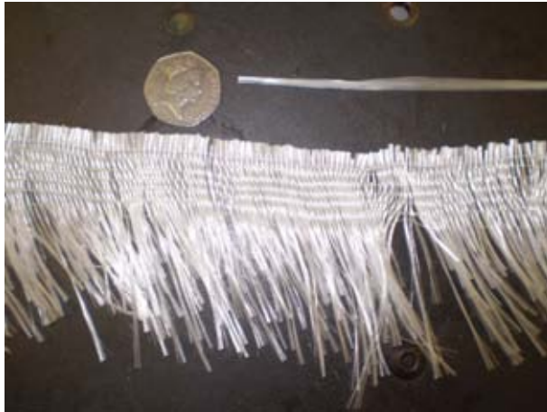
Figure 7 Photograph of DLW compared to the continuous glass fibres used in the existing clean filament winding system.
