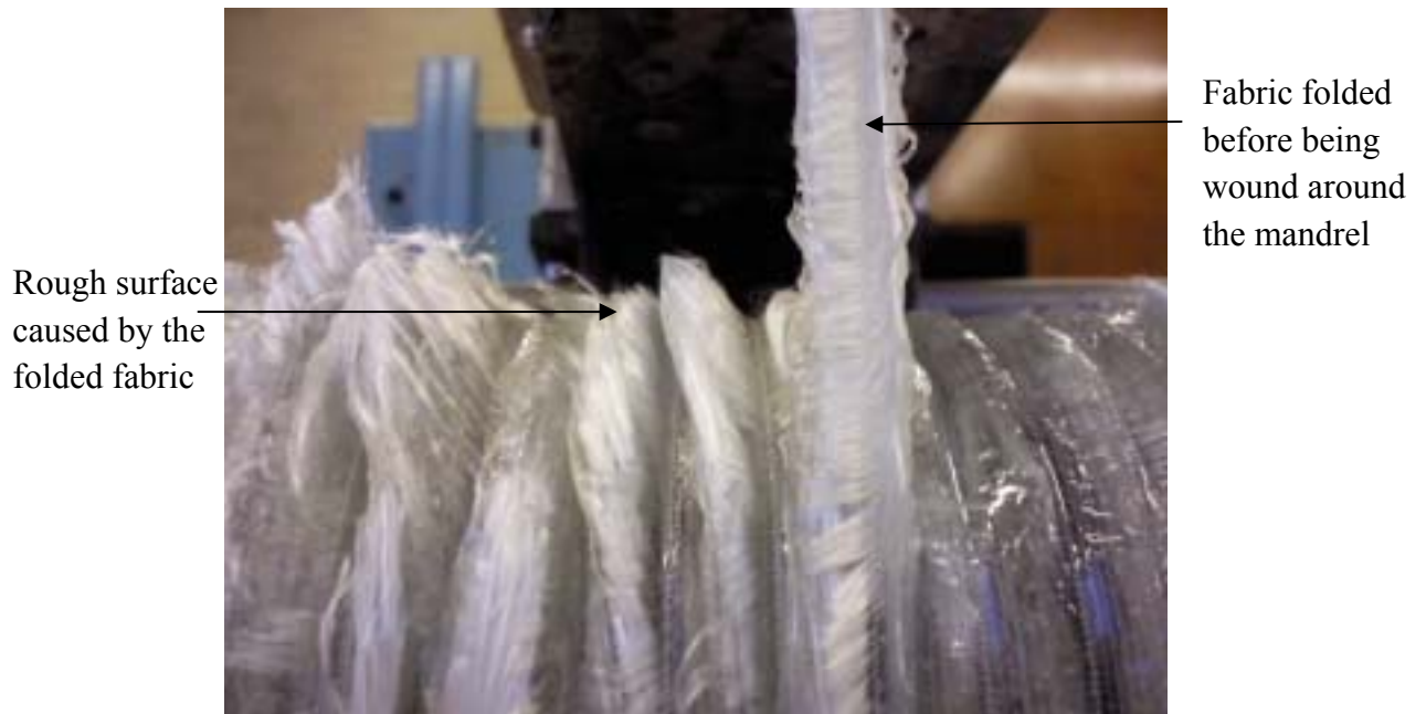
Figure 52 Photograph showing a second layer of the folded fabric being applied to the mandrel. The image demonstrates the rough surface finish caused by the folded loose edges.
