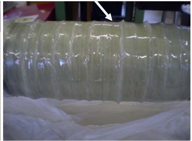
Figure 49 Photograph showing the rough surface left by the layer of continuous glass fibres.
