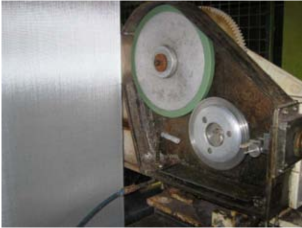
Figure 10 Photograph to show the rollers which apply the resin sealant to the edge of the glass fibre fabric.
