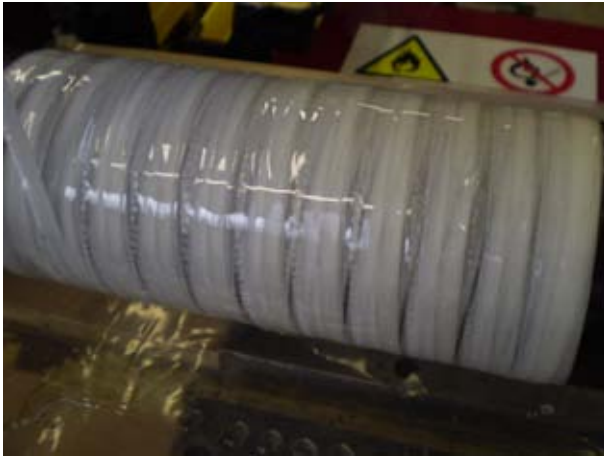
Figure 16 Photograph to show the 20mm pitch tube during the production.
