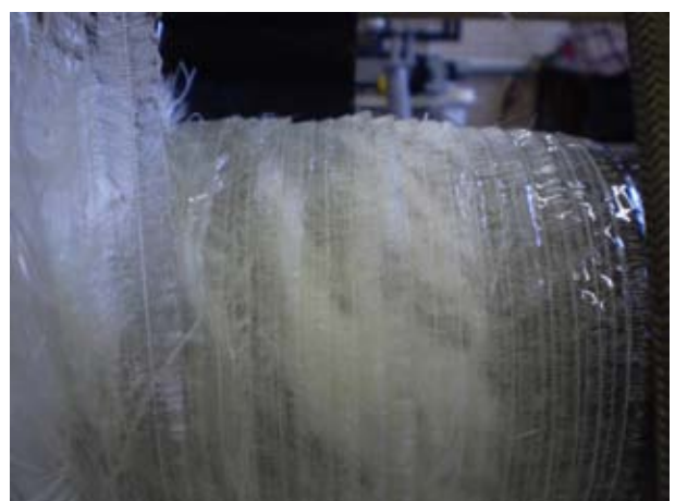
Figure 43 photograph shows the second layer of DLW being applied to the rotating mandrel trapping the loose fibres.
