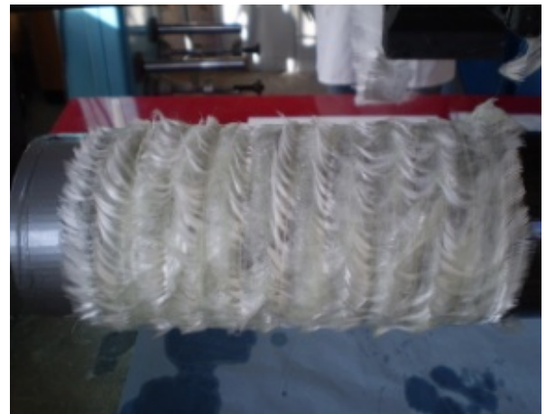
Figure 29 Photograph showing the tube produced using two layers of sewn DLW.
