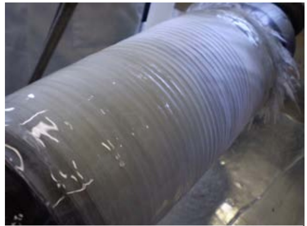
Figure 25 Photograph showing the tube produced after a layer of peel-ply has been applied to the two layers of DLW also under tension.
