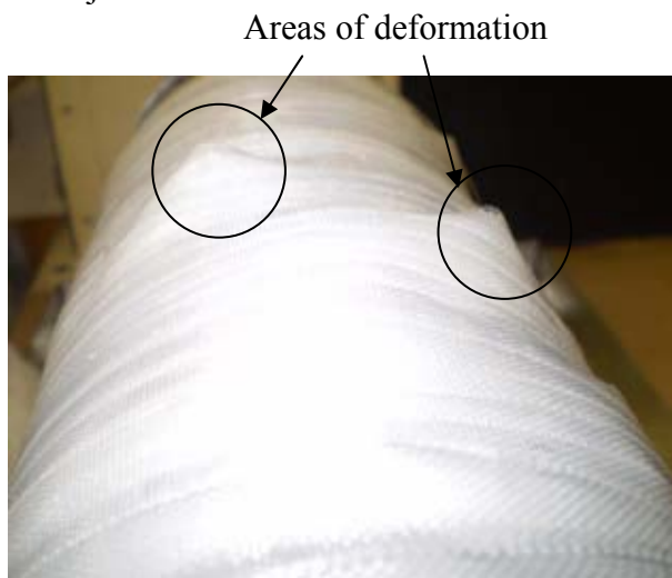
Figure 40 photograph showing a close up of the deformation (highlighted in the circles) of the fabric occurring on the tube during the winding process.
