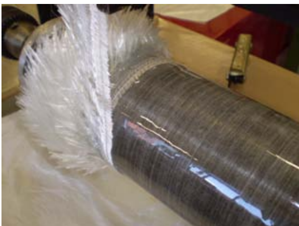
Figure 22 Photograph showing a layer of DLW being applied to a layer of virgin continuous glass fibres.
