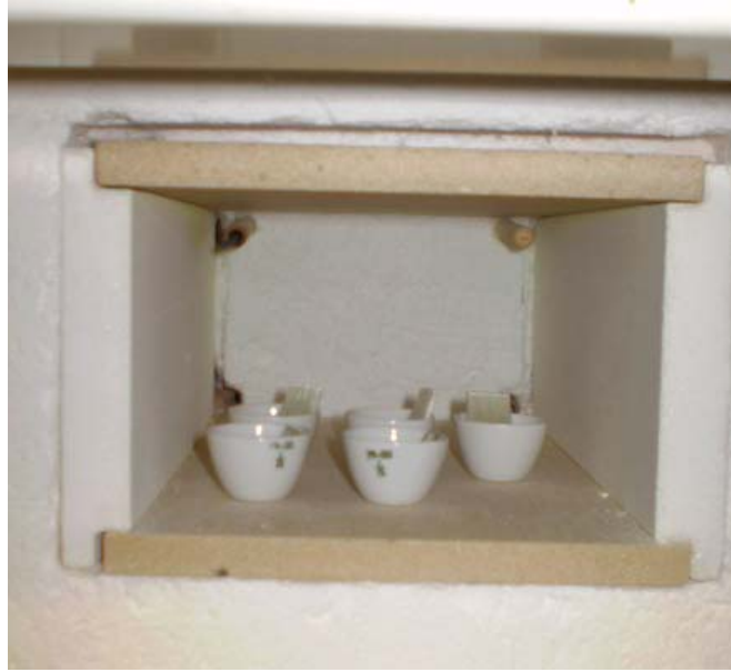
Figure 34 Photograph showing 5 samples in crucibles placed in the oven ready for the resin burn off.
