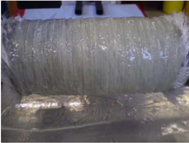
Figure 24 Photograph to show the tube produced after a second layer of DLW has been applied to the mandrel under tension.
