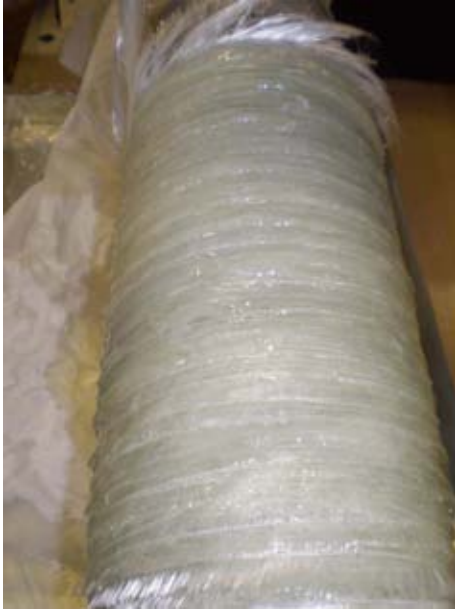
Figure 20 Photograph showing the tube produced after a second layer of DLW was applied.
