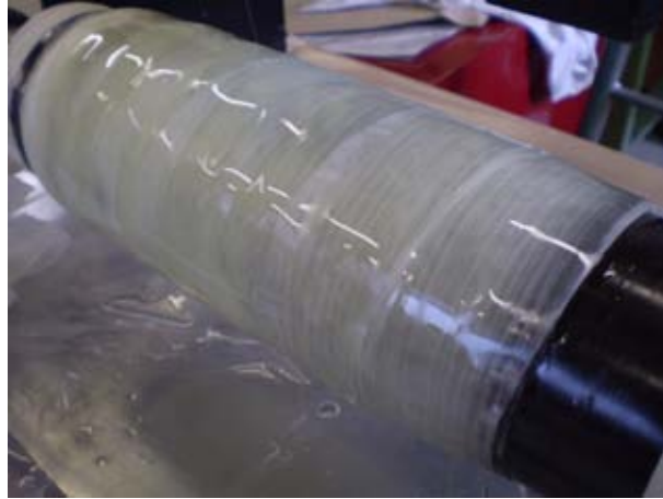
Figure 47 Photograph showing the layer of peel ply applied on top of two layers of direct loom waste. Heavily over impregnated with resin.
