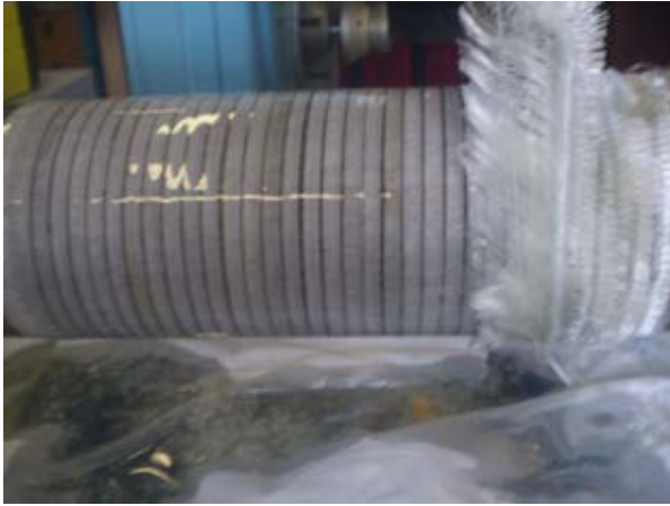
Figure 30 Photograph showing the first layer of DLW applied to a layer of the waste slittings.
