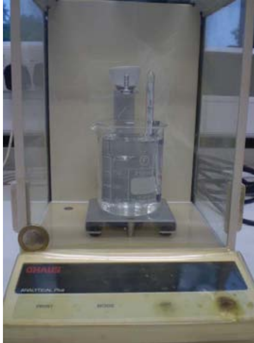
Figure 33 photograph to show the experimental set up for measuring the density of samples.
