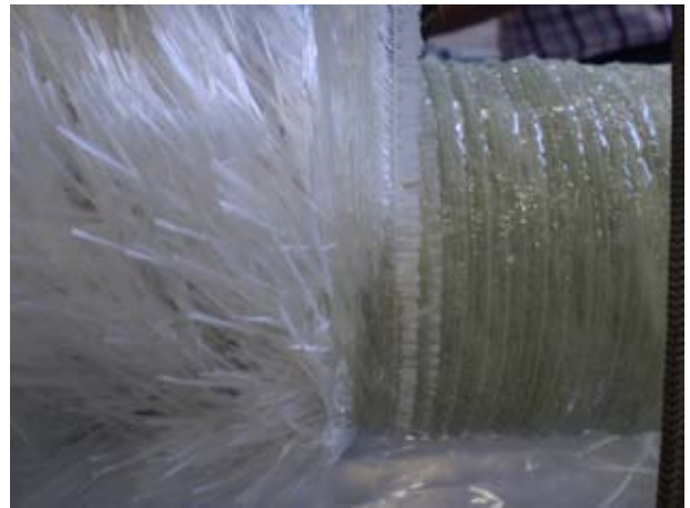
Figure 19 show the hedge hog appearance of the first layer of DLW being trapped by the second layer of DLW applied.
