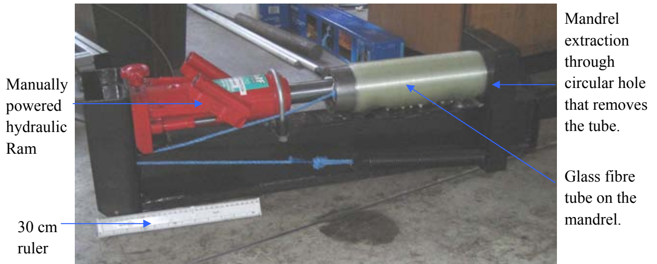
Figure 32 Photograph showing mandrel extractor system with a glass fibre filament wound tube prior to extraction.
