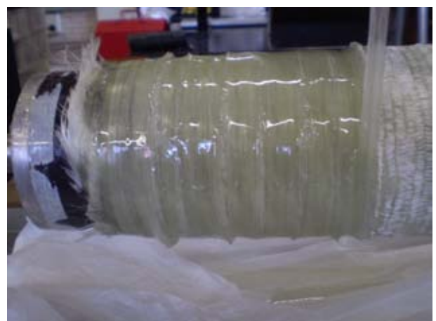
Figure 23 Photograph to show a layer of virgin continuous glass fibres being applied after two layers of DLW have been wound.
