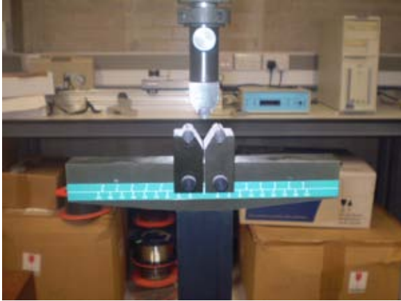
Figure 36 Photograph to shows the experimental set up for the interlaminar shear strength test
