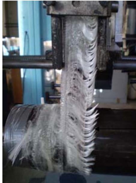
Figure 53 Photograph to show the first layer of sewn DLW being applied to the mandrels and how the loose edges have been trapped by the extra cotton thread.
