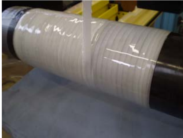
Figure 15 Photograph showing the 7 mm pitch slitting waste tube during the winding process.
