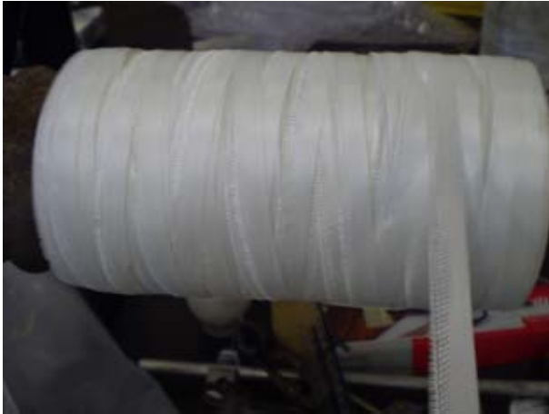
Figure 12 Photograph showing the as received waste slittings on the creel.
