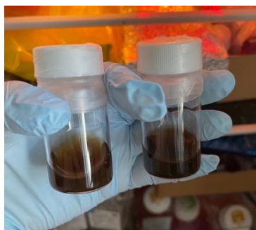
Figure S1: Digital photograph of the dispersion condition of graphene oxide dispersion after 15 minutes of sonication in a water bath. The concentration of GO shown is 1mg/mL in water.
