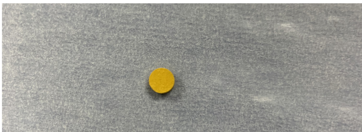
Figure B.5: Pellets of as prepared \text{RuP}_3\text{SiO}_{11} following the optimized method using \text{Ru}(\text{PO}_3)_3 as a starting reagent.
