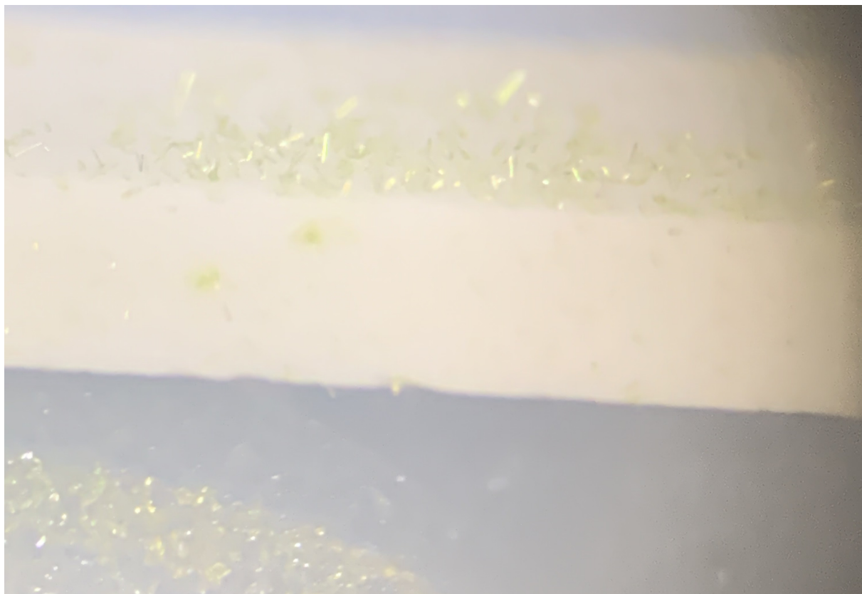
Figure B.2: Needle-like single crystals of KMP forming on the walls of the boat crucible.
