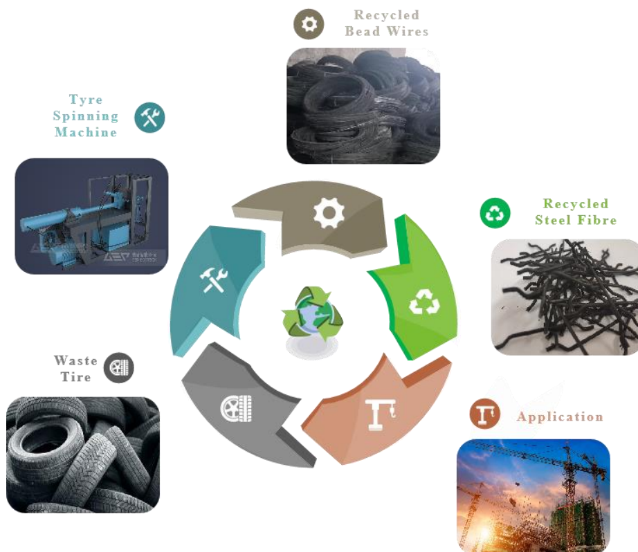
Figure 6-1 Manufacturing process of RSF
