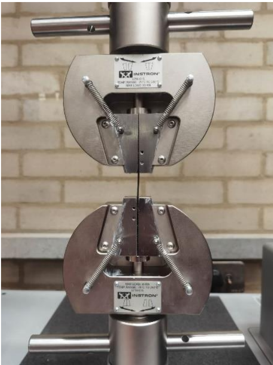
Figure 3-2 Fibre tensile strength test
