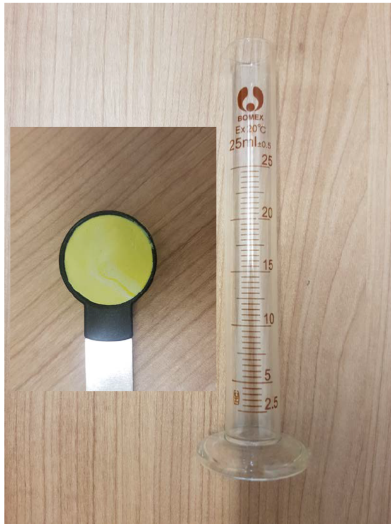
Figure 3.3 Left: Measuring spoon used to measure 2\text{cm}^3 of putty - simulated volume (explant) of known volume. Right: 0.5ml gradient measuring cylinder used for the water displacement technique to validate the gold standard volume of putty.
