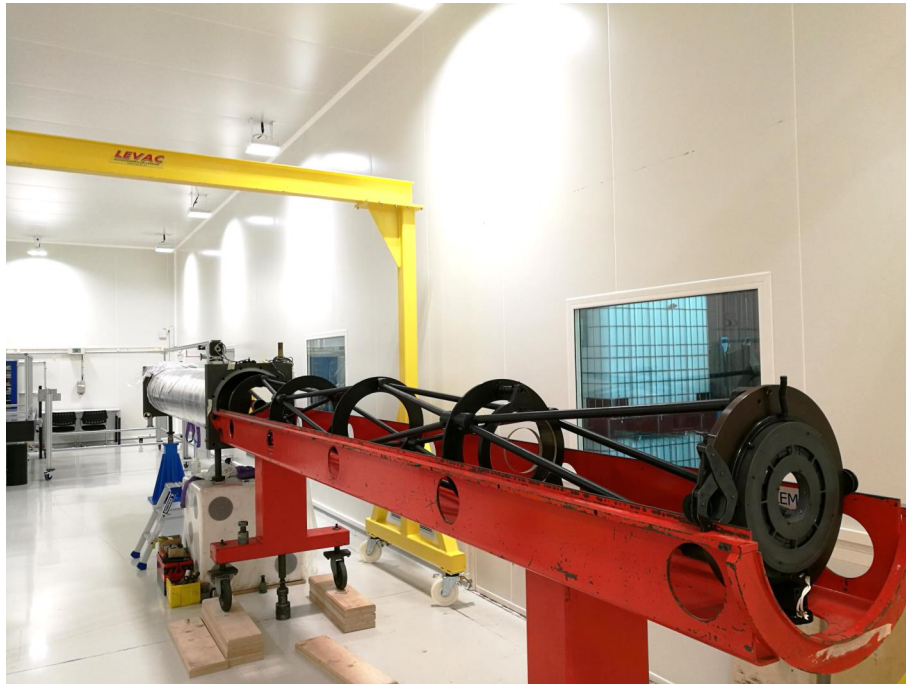
Figure A.2: An opened CEDAR (photograph taken by Serge Mathot (CERN)).
