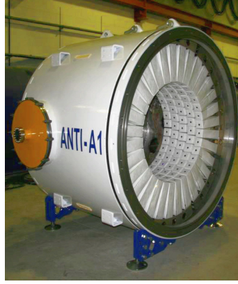
Figure 2.13: The first LArV station before placement in the vacuum vessel. Image reproduced from Ref. [67].
