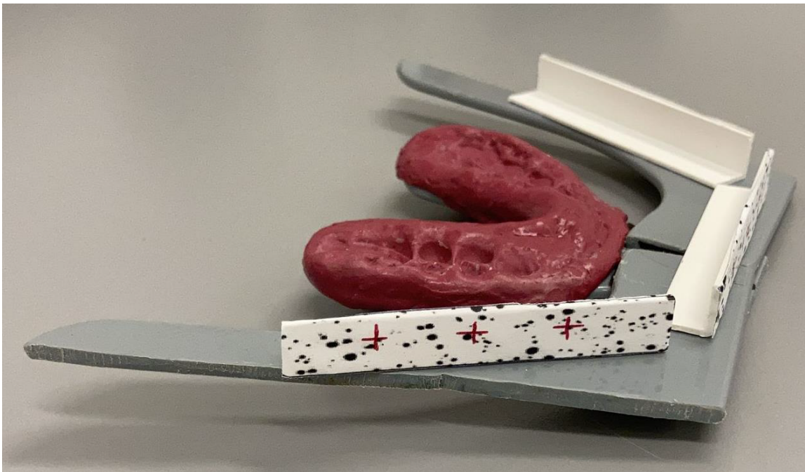
Figure 3.2 3DMOD showing speckled paper application and red cross-hair landmarks.
