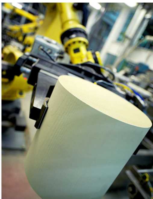
Figure I-4: Monolith used in the production of a catalytic converter for vehicle emission control ( https://matthey.com ).
