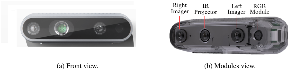
Figure 4.3: The intel Realsense D435 camera contains RGB module and depth module (IR projector, left & right imagers).
