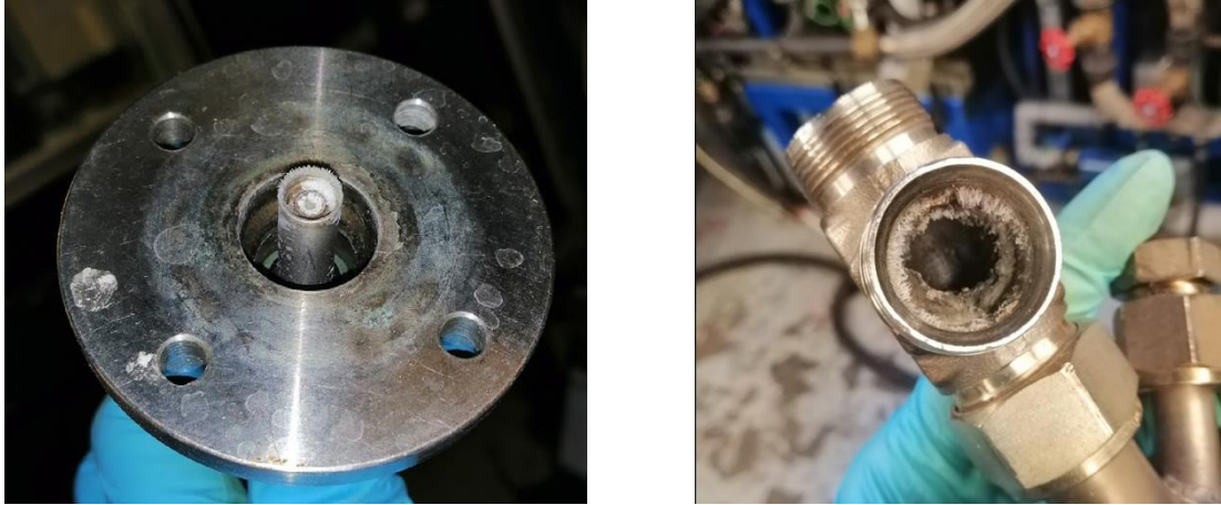
Figure 2-2: Urea solid deposit on the injector nozzle (Left) and on tube wall of laboratory-scale mixing chamber (Right)
