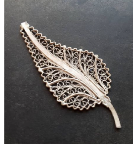
Figure 1.2. An example of the creation of a filigree motif (a leaf). A: The outer framework of the leaf is made from thicker wire. B: A thinner skeleton is used on the inside. C: This is then filled with coils or finely twisted wire (kindly provided by Charmaine Gerada)
