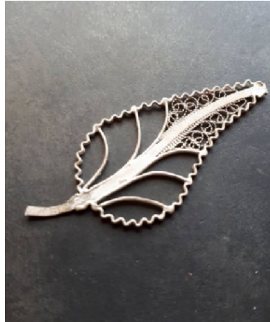
Figure 1.2. An example of the creation of a filigree motif (a leaf). A: The outer framework of the leaf is made from thicker wire. B: A thinner skeleton is used on the inside. C: This is then filled with coils or finely twisted wire (kindly provided by Charmaine Gerada)
