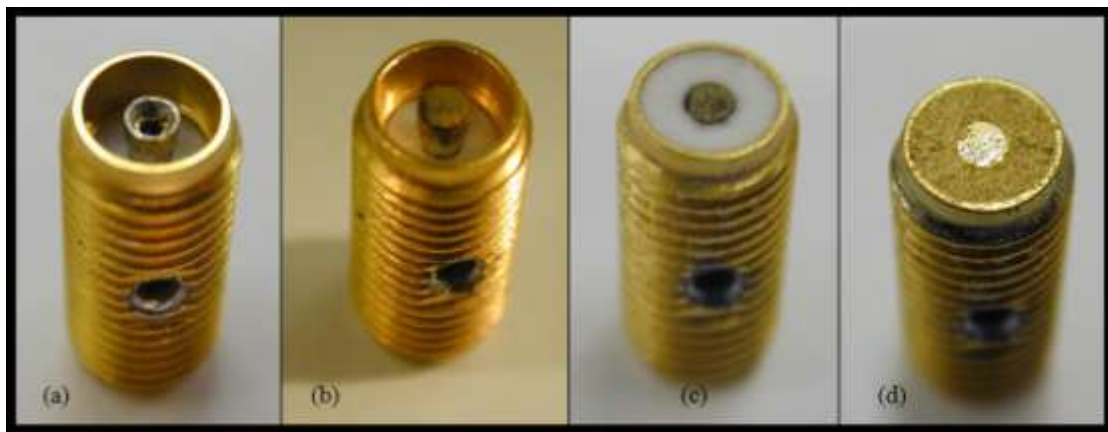
Figure 7.2 (a) Modified SMA connector with socket pin (b) Composite disc mounted on socket pin (c) After potting with insulating epoxy/glass micro-balloons (d) Complete transducer with ground Au electrode applied
