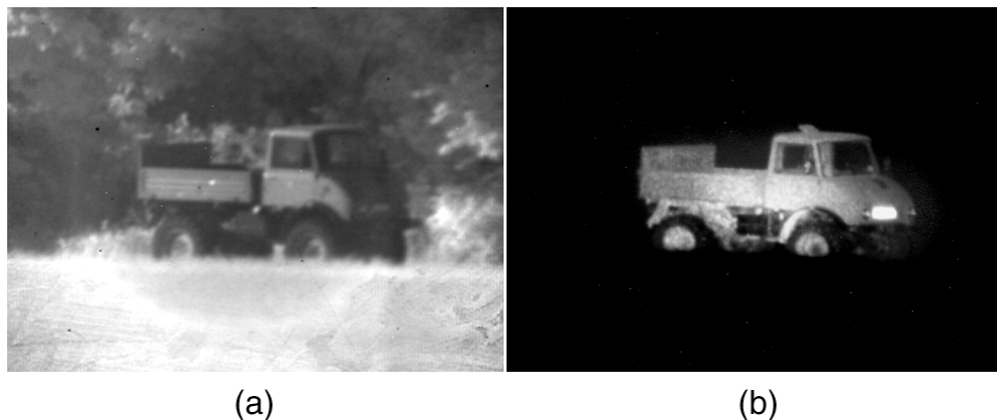
Figure 2.12: SWIR passive (a) and SWIR gated imaging system (b) images at a range of 480m. This technology allows for isolating elements of a scene and the improvement in clarity due to reduction in backscattered photons. From [2].
