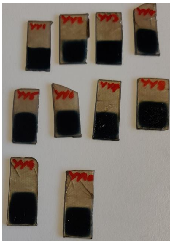
Figure 6-14: PEDOT:PSS/Tween 80 dip cast film samples on PET/PDA substrates used for adhesion scratch testing. Surfactant concentration increases with increasing sample number
