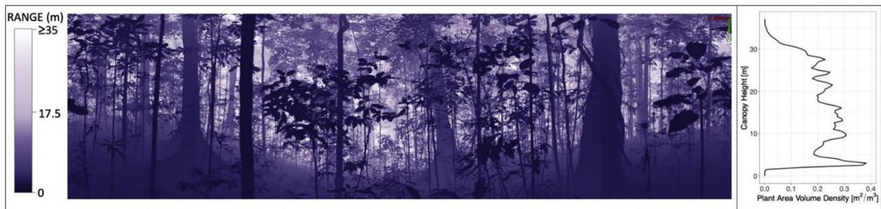
3140 Figure 5.9: 3D complexity of a Simple Notophyll Vine Forest (Robson Creek, Australia) captured using a time-of-flight RIEGL VZ-400 instrument. Left panel: The colours represent the distance from the scanner. Right panel: Derived plant area volume density as a function of canopy height derived for the same scan using (Calders et al. 2015). Figure and caption reproduced without modification from Calderys et al. (2020) under Creative Commons License CC BY 4.0. ‘Plant area volume density’ refers to PAD.
