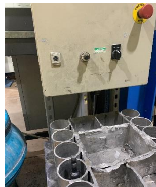
Figure 3.3: Vibratory station to tap powder filled canisters
