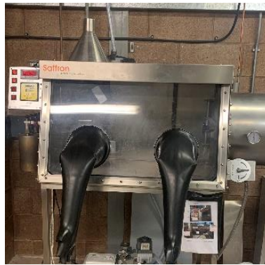
Figure 9: Glovebox used to fill powders photograph
