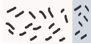
Figure 2.1: Discontinuously reinforced MMC (a-b), [10]
