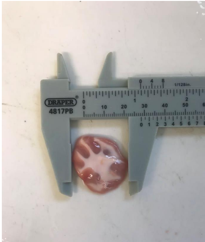
Figure 3.2 – A representative image of a test brain specimen. The dimension of each specimen was measured before mechanical testing.
