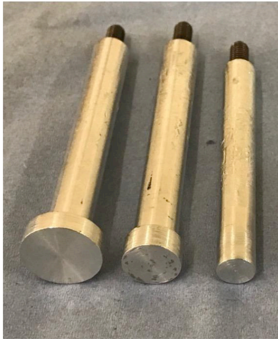
Figure 3.4 – Three circular flat indenters with diameters of 16 mm, 12 mm and 8 mm.
