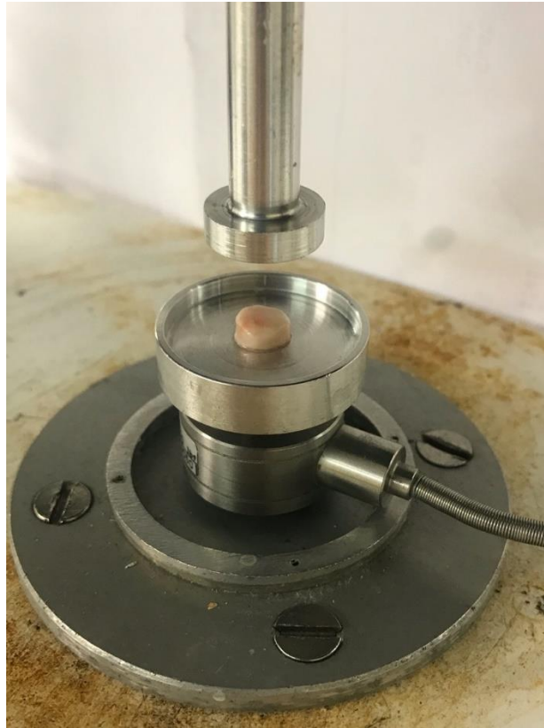
Figure 4.5 – Experimental setup for the compressive DMA of bovine brain tissue specimens.
