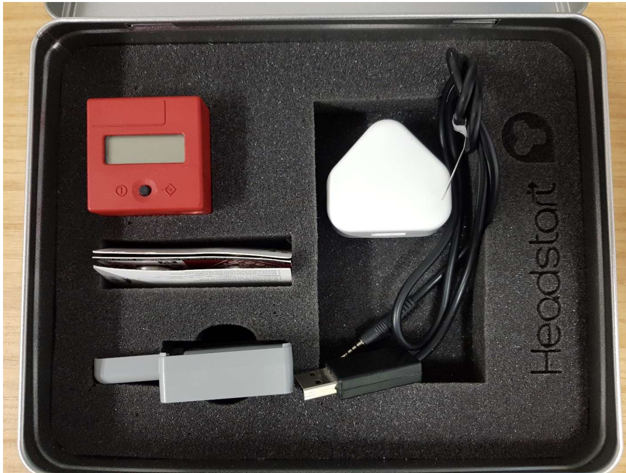
Figure 2.7: Lateral flow assay cube reader (red), base plate (grey), connect wire (black) and plug (white) with spare batteries
