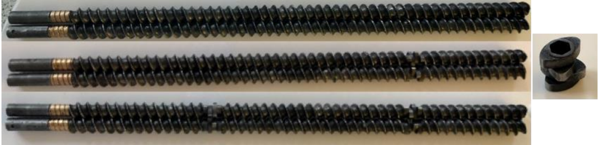
Figure 3-2 The screw configurations used within the study: conveying elements only (C), 1 kneading zone (1K) and 2 kneading zones (2K). The picture to the right shows a single 60° kneading zone.
