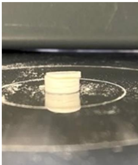
Figure 7-3 Demonstrating the failure of MCC tablets produced from material containing 2% w/w MgSt and stored at 75% RH.
