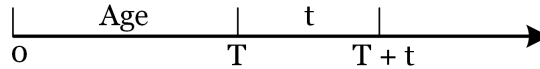
FIGURE 3.4: Diagram used to explain the concept of probability of transition to ageing failure [17]
