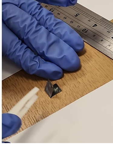
(b) Folding the Al foil around the Eu foils.
