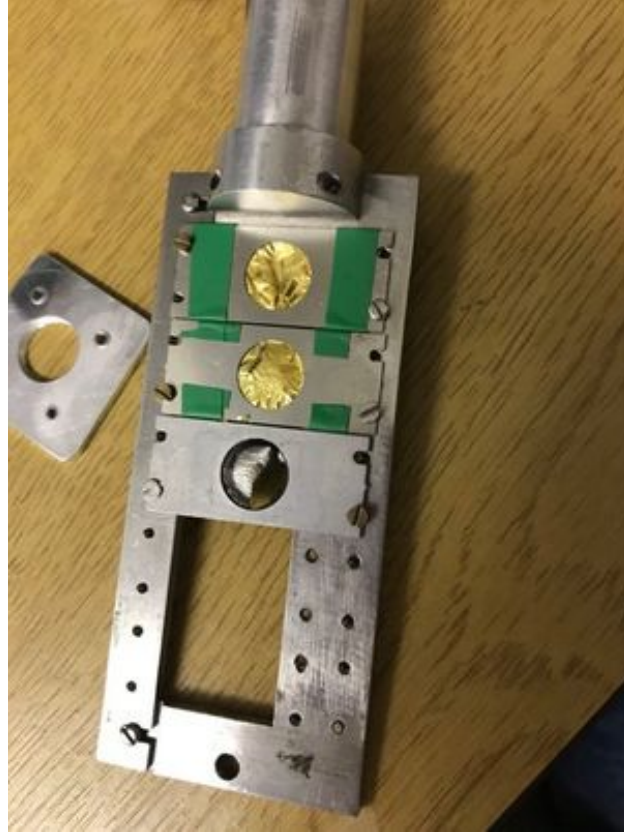
Figure 3.13: Target ladder with two gold foils the top is 300 \mu\text{g}/\text{cm}^2 thick and the second one below is 200 \mu\text{g}/\text{cm}^2 thick.
