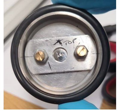
(c) Final stack of foils in target holder.
