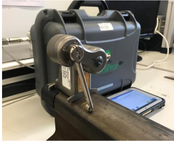
Fig. 5.23. MiniProf full-contact rail profile measurement system
