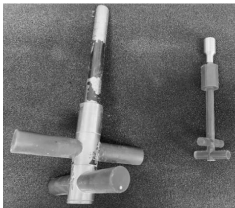
Figure 3.5: Lab-Scale Impeller (left) and 3D Printed Impeller (right)
