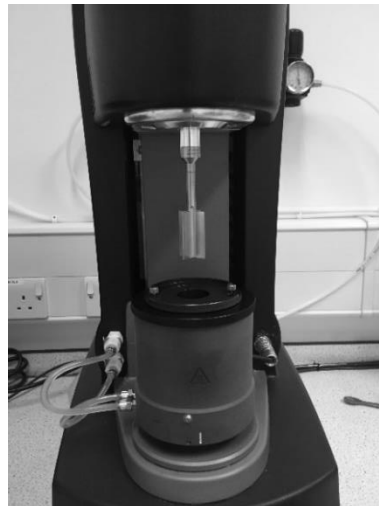
Figure 3.6: Vane Rheometer Geometry with Trios Rheometer
