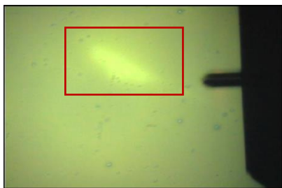
Figure 10.7. Optical microscope image of the bloom region (framed) in a plasticised PVA film containing 3 wt% CTAB after two months of sample storage. The length of the protruding cantilever is ca. 125 \mu\text{m} .
