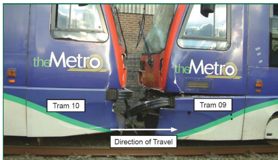
Figure 41: Trams 10 and 09 after the Collision (RAIB, 2006)
