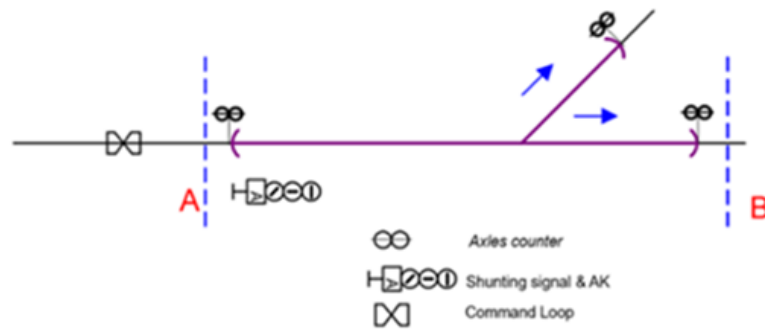
Figure 28: Controlled Section (ALSTOM, 2008a)
