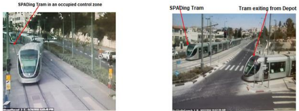
Figure 29: Potential for Collision between Trams in Controlled Sections
