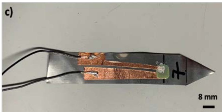
Figure 5.10 Schematic graph of the bulk energy harvester, a) side view, b) top view and c) final prototype of cantilever energy harvester
