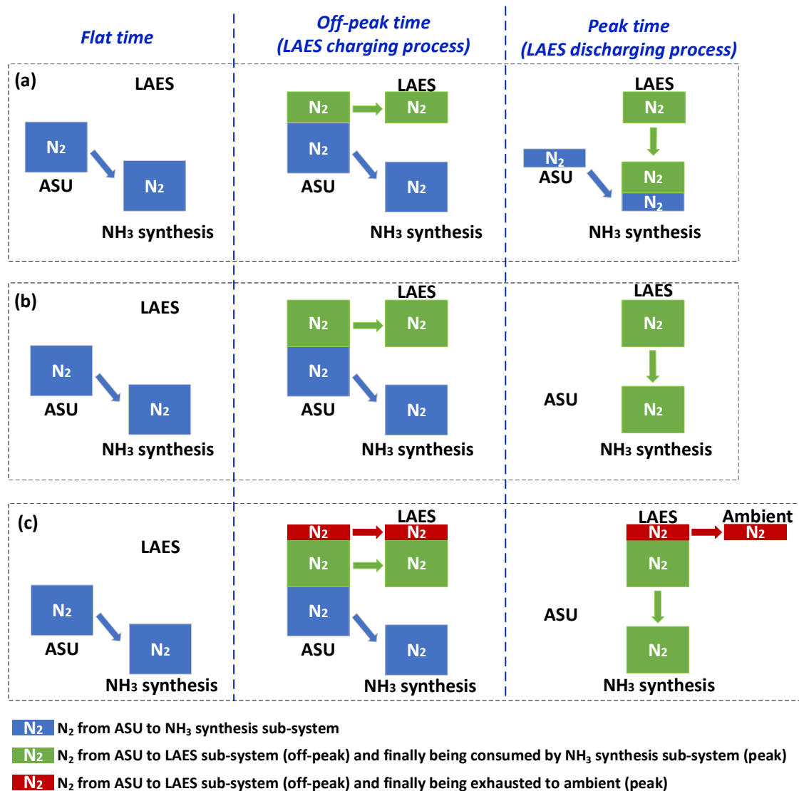
Figure 7.8 Three operation modes of the LAES-NH 3 system: mode (a), (b) and (c).
