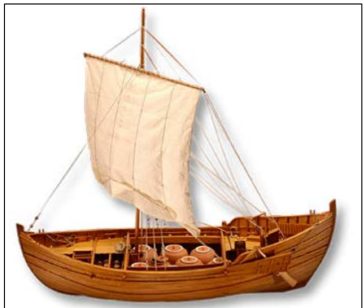
Fig. 2.5. Model of a dolia ship based on various shipwreck finds (Centre Camille Jullian).
