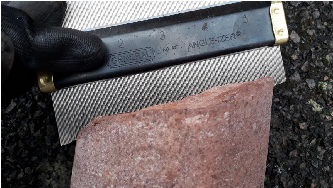
Figure C-5 Use of a profile gauge on a joint surface of Kelly Burn Sandstone.
