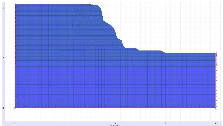
Figure D-23 Excavation to 10 mOD following the quarry profile.
