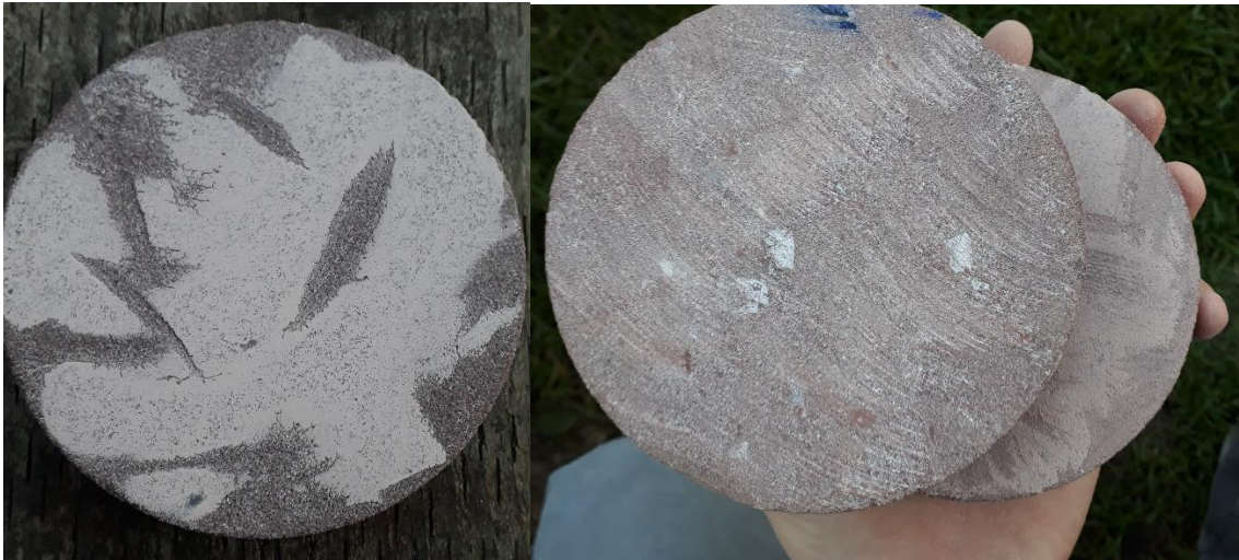
Figure 7-5 Preparation of discs for sliding tests.
