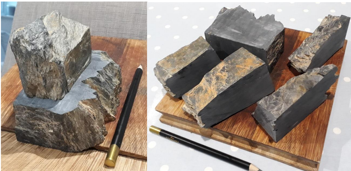
Figure 8-19 Prepared block samples and sliding test (left).
