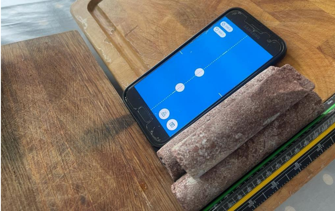
Figure 7-4 Small scale tilt tests on Kelly Burn Sandstone with inclinometer.
