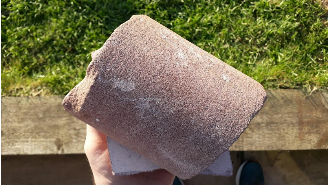
Figure 7-7 Preparation of axially cut cores for tilt testing.
