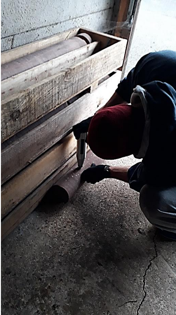
Figure C-3 Schmidt hammer testing of core material.
